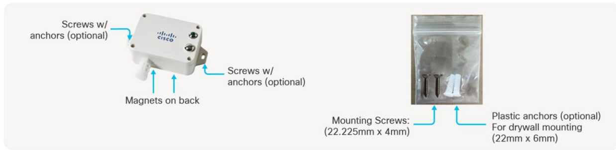
Figure 7. Mounting Accessories and Methods AV201
