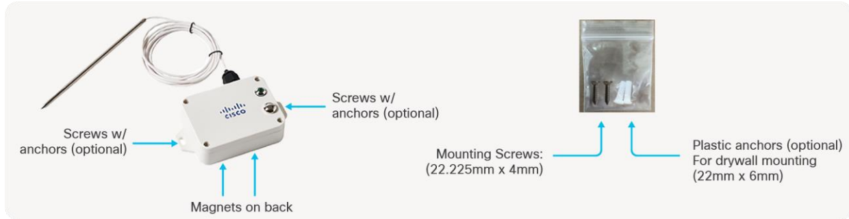
Figure 10. Mounting Accessories and Methods AV202
