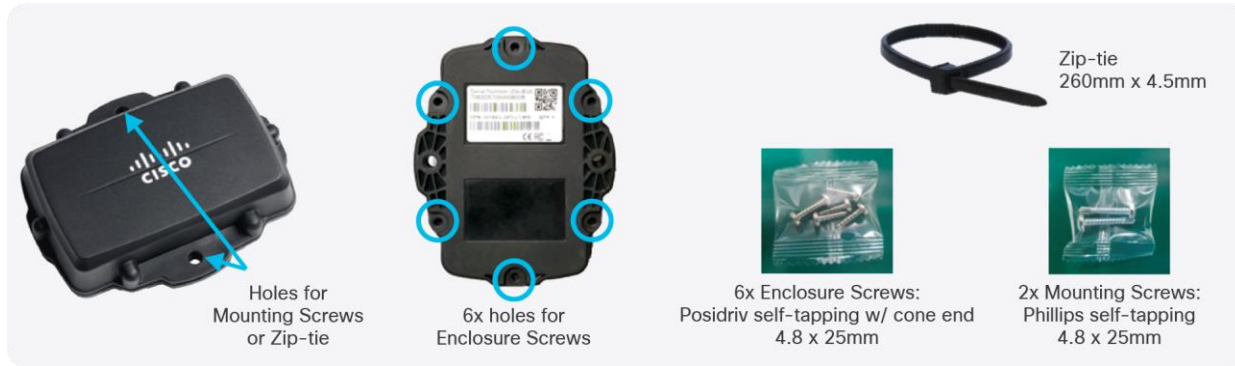
Figure 33. Mounting Accessories and Methods AV300
