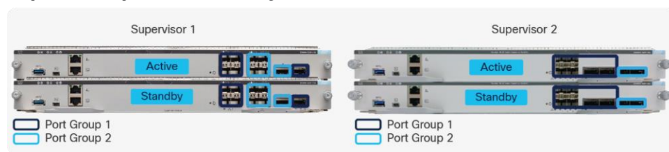
Figure 36. Dual supervisor uplink configurations
